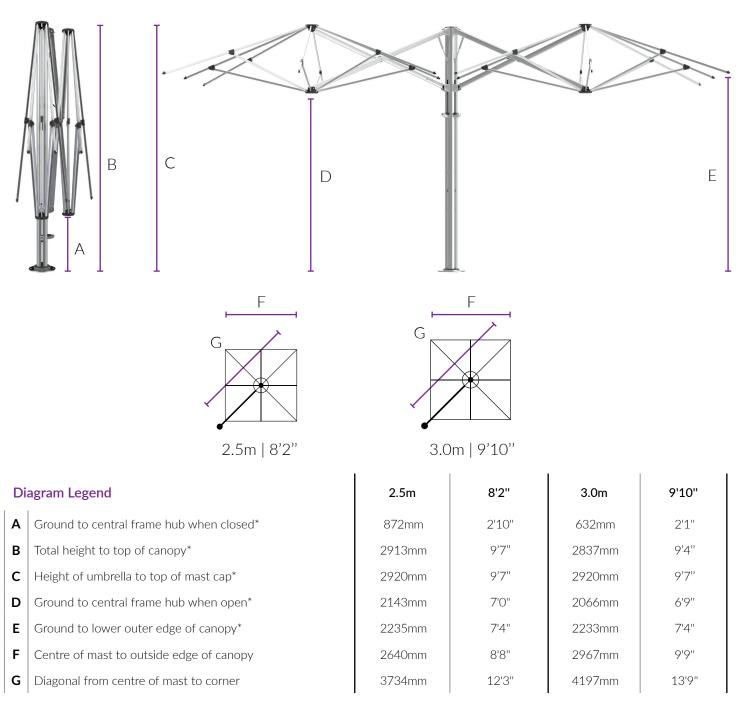
\*Free-Standing base installations will add 165mm | 6" to the height and surface plates will add 12mm | ½" to the height. Adding Free-Standing Base wheels also will add a further 45-80mm | 2-3". All sizings are +/- 2.5mm |  $\frac{3}{22}$ " and subject to change without notice.
